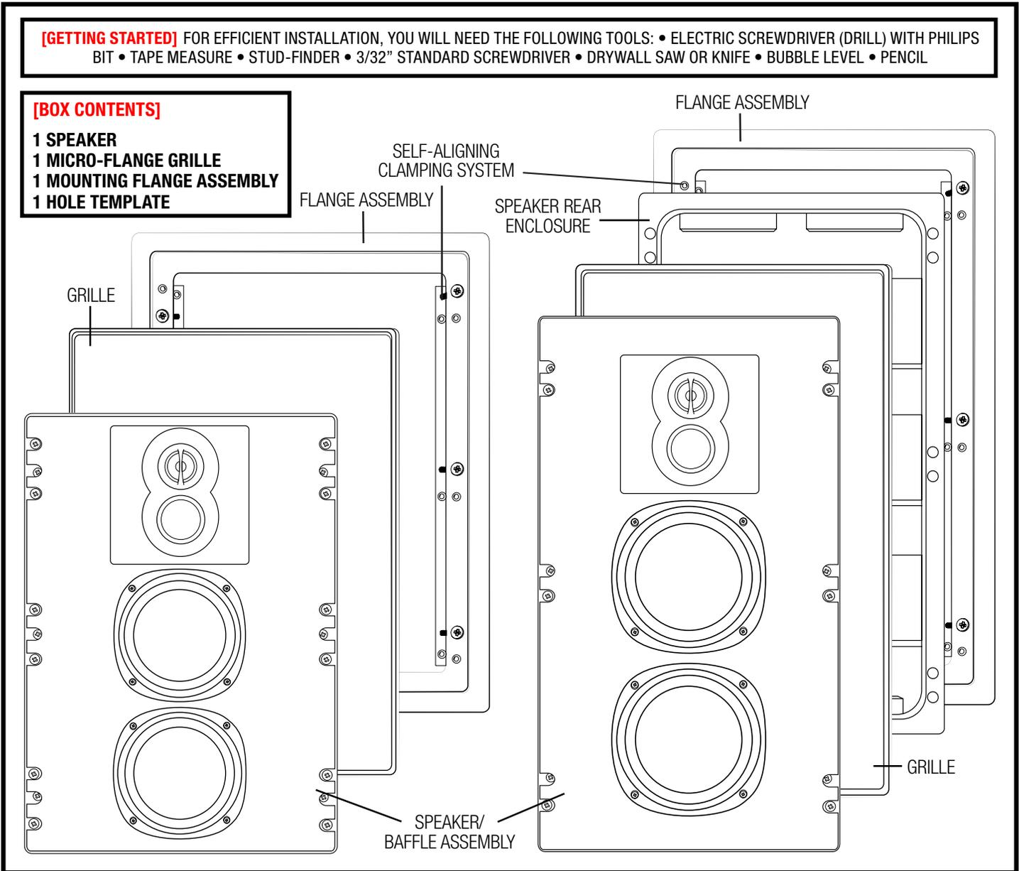
Thank you for purchasing the Phase Technology<sup>®</sup> CI Custom Installation high definition in-wall speaker system. The mounting frame of extruded aluminum has a uniquely designed self-aligning clamping system to secure the flange assembly to the drywall. This patented design simplifies installation and reduces unwanted wall vibration resulting in improved performance and definition.
